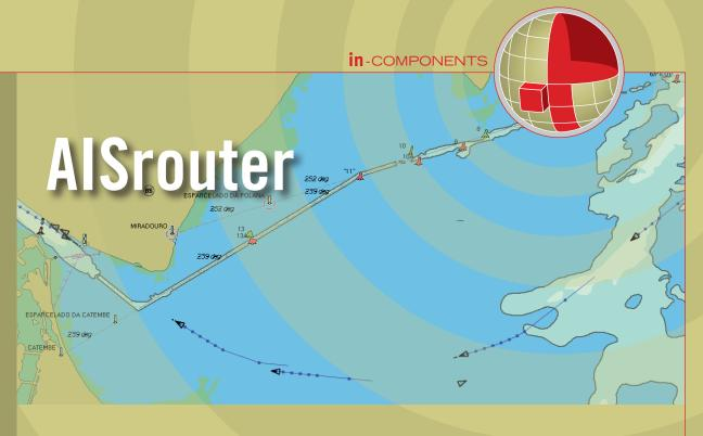
In AIS networks with several base stations, the AISrouter ensures that AIS data are forwarded from land to ship using the most efficient way possible.
