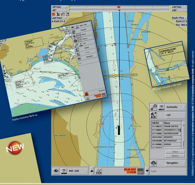
Display of electronic charts is standard equipment in inland navigation. **RADAR** *pilot720° info* provides this basic functionality. However, AIS information is indicated, additionally.
